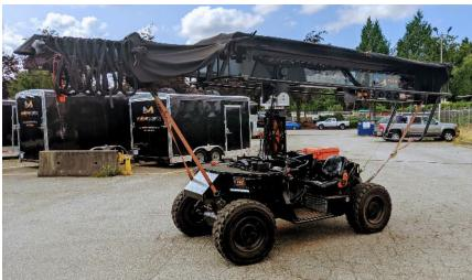
The BADGER diesel-powered motorized base uses a hydraulic drive system with the ability to steer in standard, crab or round on either rubber-tired wheels or tracks. The self-leveling post system and no need for outriggers allow for faster setup time and maximum arm swing clearance.
